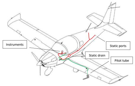
Keep the pitot head clean to ensure proper functioning of the system. Ensure that the Pitot tube cover is removed prior to every flight and that it is replaced after every flight. Check the static ports on both side of the fuselage for any obstructions before every flights.
