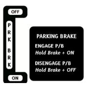
On the spacing panel between the cockpit and baggage area 1:
