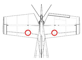
It is also acceptable to push the aircraft carefully backwards by putting pressure on the wing leading edges close to the root, directly on a nose rib, or on the horizontal stabilizer leading edge next to the root over a rib.
