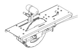
A trim level indicator is provided left of the actuation wheel, indicating on a mobile scale the current trim tab position.
