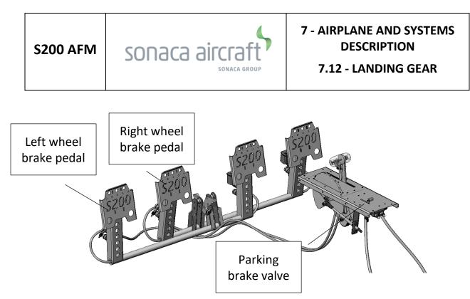
To actuate the brakes using pedals, apply pressure on the top of each pedals using your toes. This will rotate the pedals around their central axis, and compress the two brakes cylinders.
