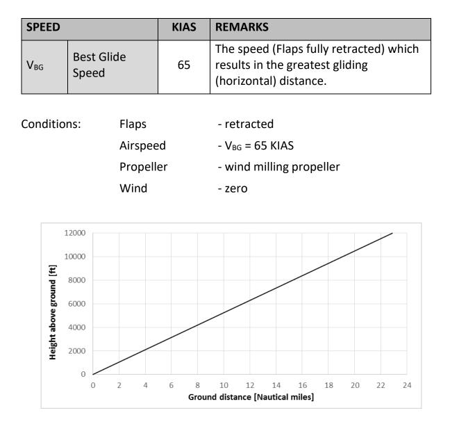
Horizontal distance travelled (still air) is approximately 1.9 Nmi (3.5 km) per 1000 ft (305 m) descent (i.e. glide ratio of 11.6 : 1).
