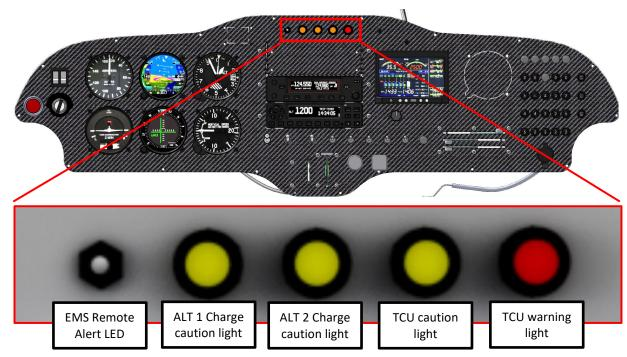
All warning lights except the EMS RAL can be dimmed by turning the light housing and can be tested by pushing on them.
